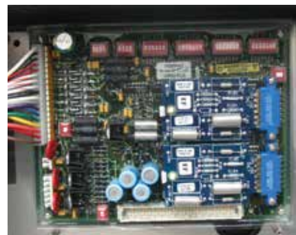
Figure 7. Typical Tri-Phase with ground trip control (TPG) module.
