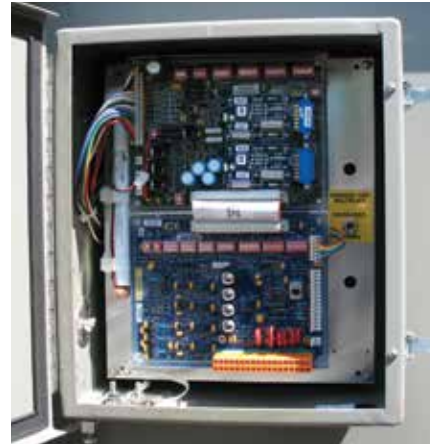
Figure 5. TPG control with SCADA shown.
